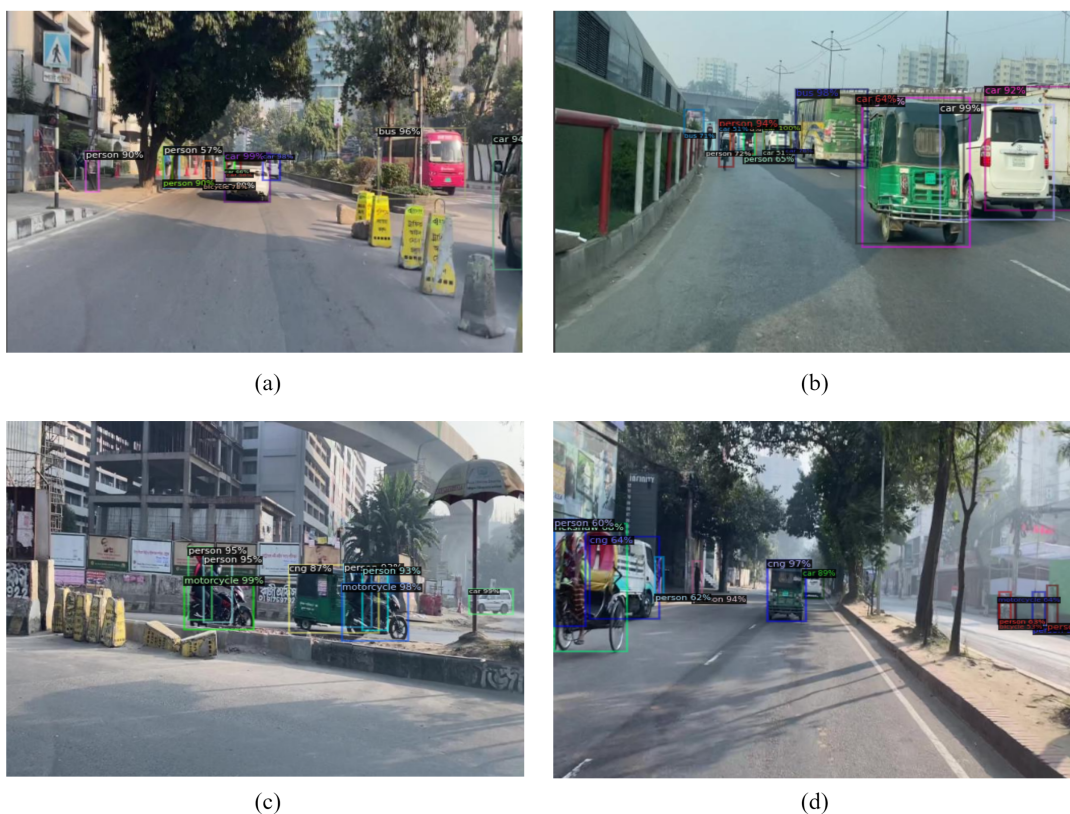
Figure 5.6: Example of occluded objects detected by Faster R-CNN on four test set images
