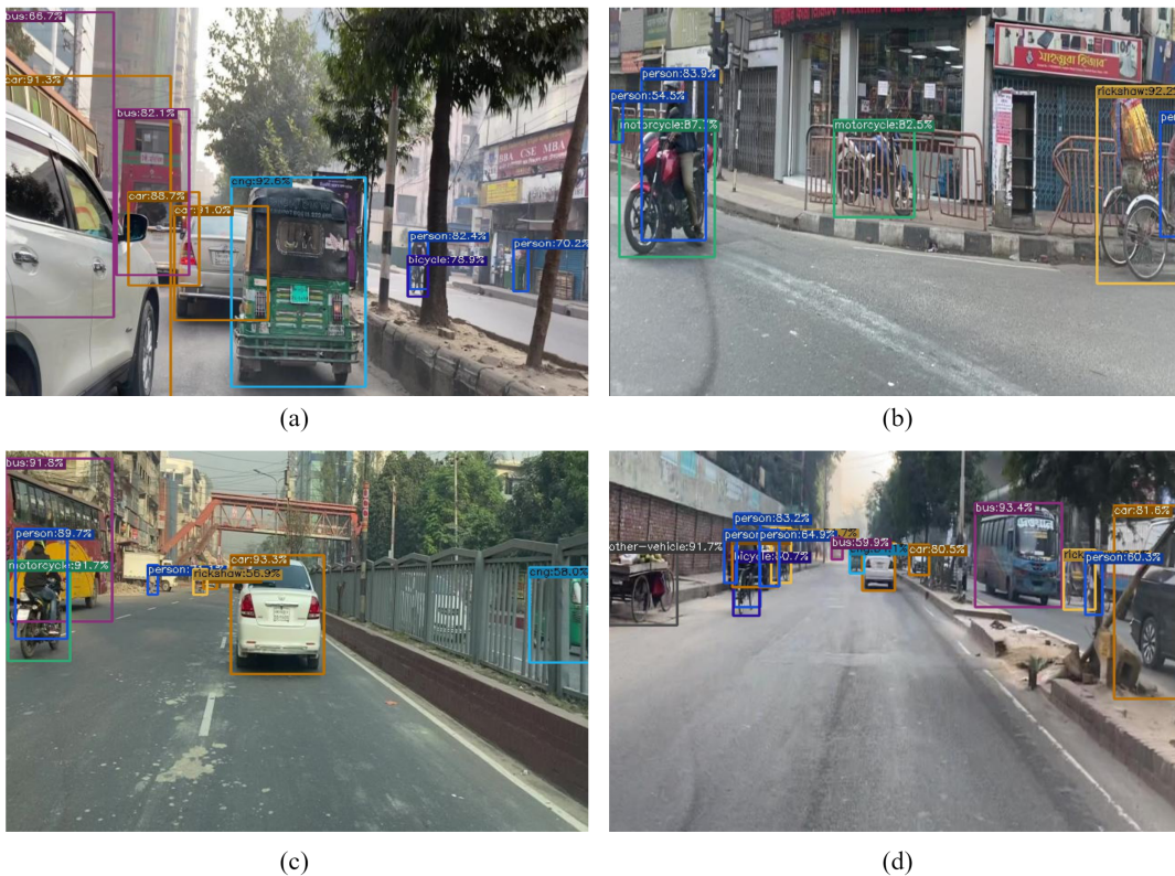
Figure 5.4: Example of occluded objects detected by YOLOX on four test set images
