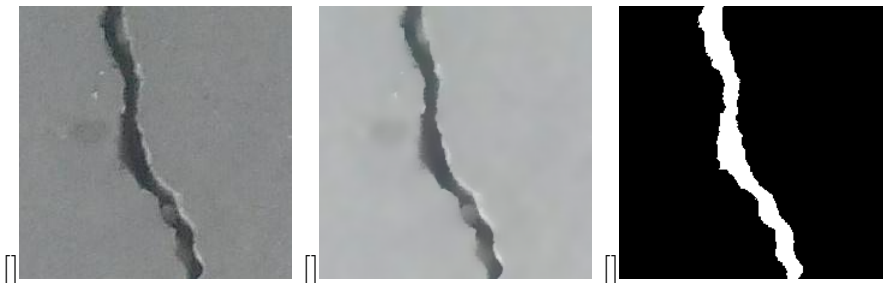
Figure 4.4: Bilateral filtering and image segmentation;(a) original picture; (b) filtered positive; (c) segmented picture.
