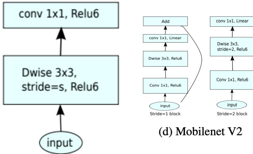
Figure 4.5: Basic layers of MobileNet and MobileNet V2 [13]
