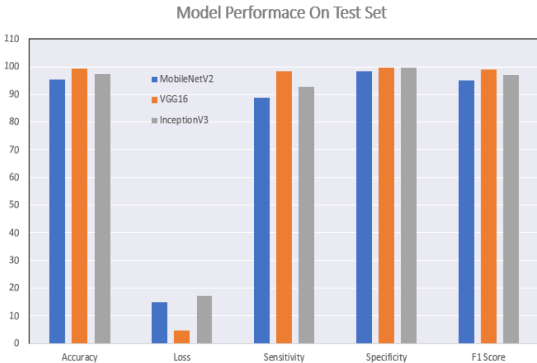
Figure 4.14: Test Performance of Different Classification Models.
