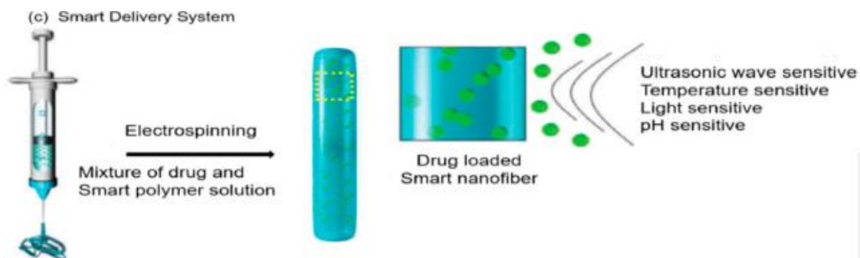
Figure 8: Smart delivery systems (stimuli responsive) (adapted from Shahriar et al., 2019)
