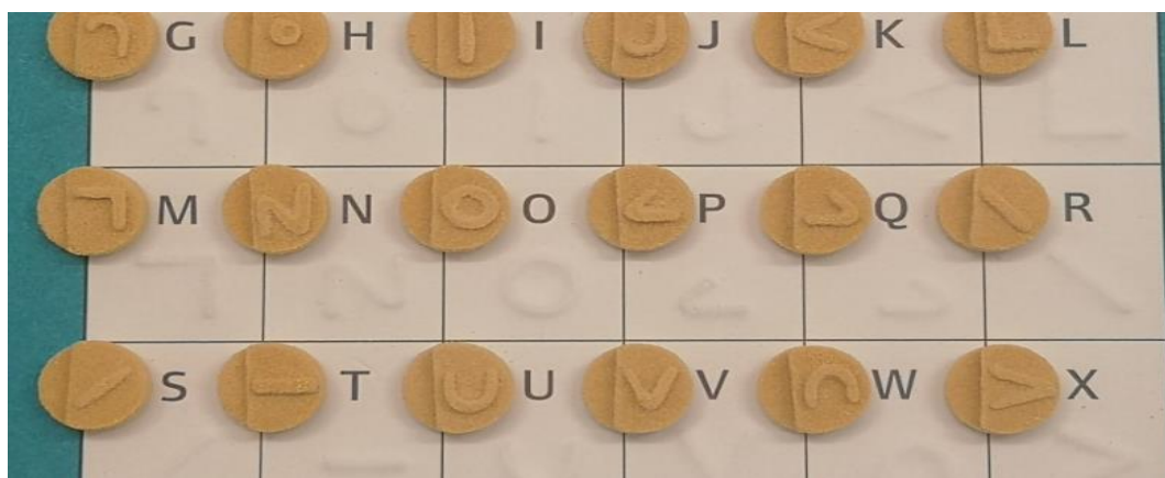
Figure 6: Illustration of cylindrical printlets comprising the 26 Moon alphabets (Awad et al., 2020)
