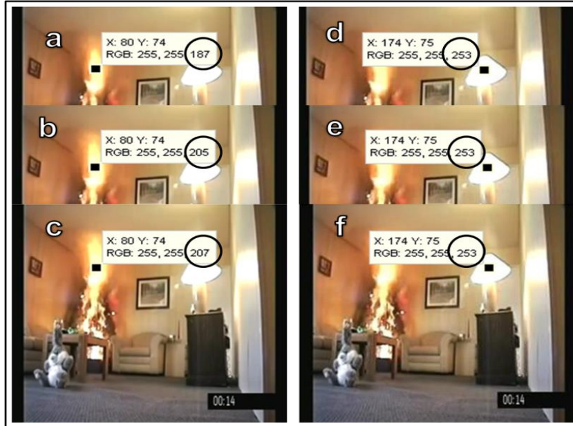
Figure 10: Variation of Blue Component Values in the Static Objects and Fire between Frames.
