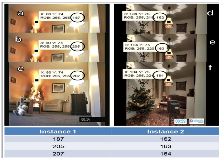
Figure 11: Tabulating the Change in Blue Component Values. (a), (b), (c) are three consecutive frames of one instance and similarly (d), (e) and (f) are consecutive frames of a second instance. Each column belongs to an instance and the three rows hold the Blue Component measures of the three frames respectively.
