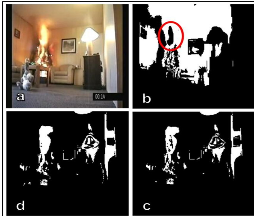
Figure 9: Color Segmentation Output by the Proposed Rules in and the State of Art Models. (a) Sample frame (b) Color Segmentation on YCbCr Using Equations (4-7) (c) Color Segmentation on RGB Using Equations (1-3) (d) Segmentation Using Proposed Equations.
