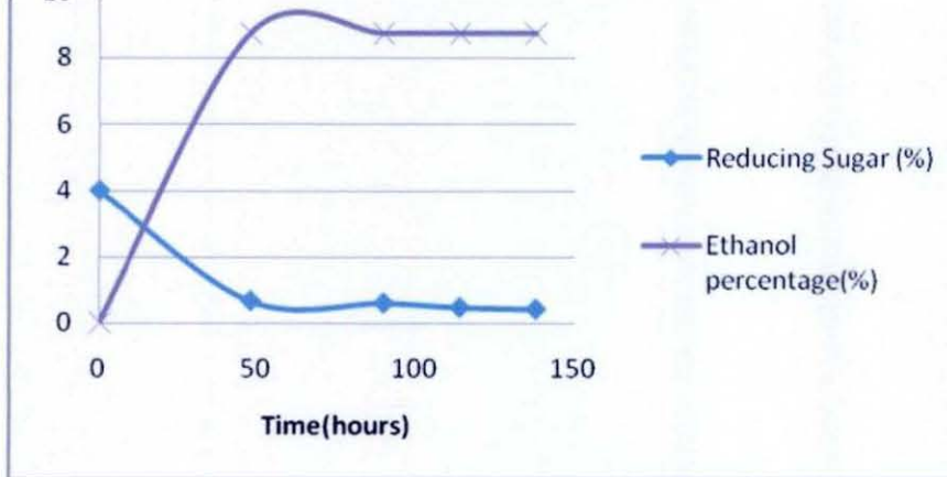
Fig-19: Production of ethanol using initial reducing sugar concentration 4.0% at 30°C under non shaking condition.
