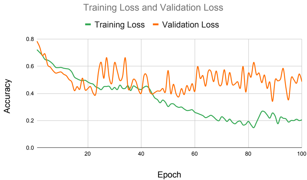
(b) Comparison between training and validation loss of MDCN (V2) on RWF-2000 dataset.
