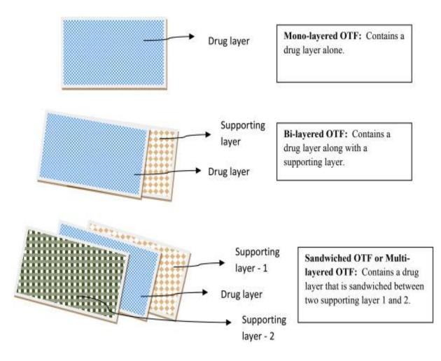
Figure 3: Classification of OTFs based on number of thin layers (Gupta et al., 2020)
