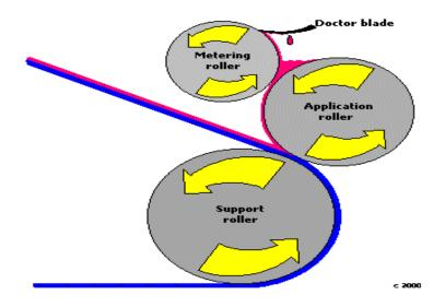
*Figure 6: Three roller coating films forming the unit (Bhusnure et al., 2017)* In figure 6, a diagram of forming film using the rolling method is given.
