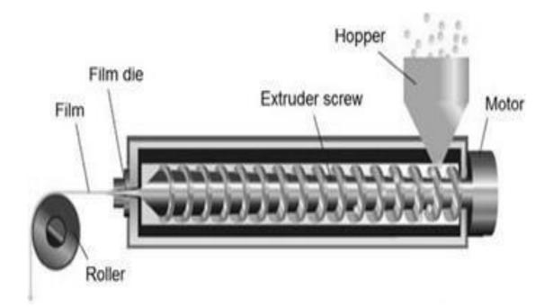
Figure 5: Hot melt extraction machine (Thakur & Tyagi, 2019)
