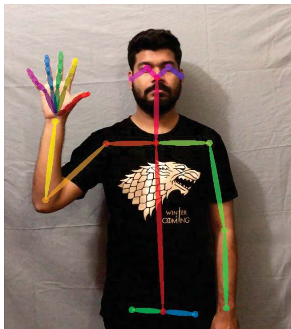
Figure 4.15: 57 keypoints of each frame.
