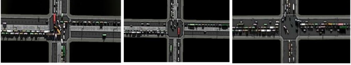
Figure 2.1: a. lane without traffic lighted left turn b. lane with traffic lighted left turn c. lane with dedicated left turn d left turn
