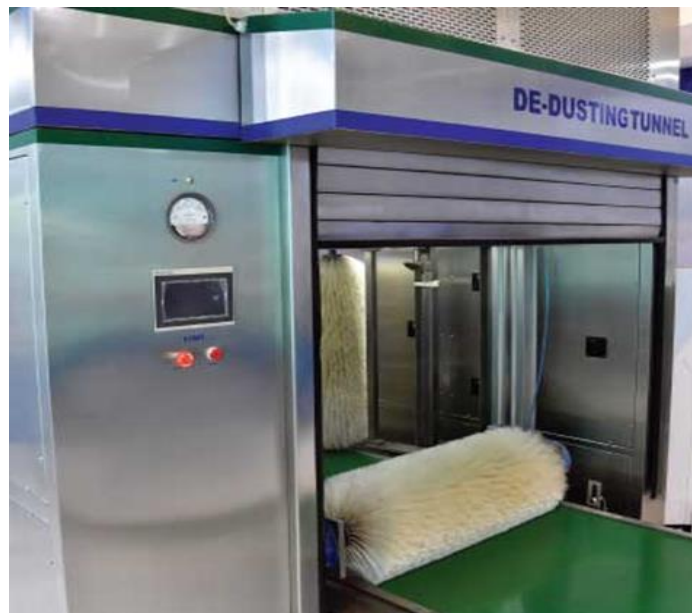
Figure 16: Fabtech De-dusting tunnel from Germany (Fabtech, 2018)
