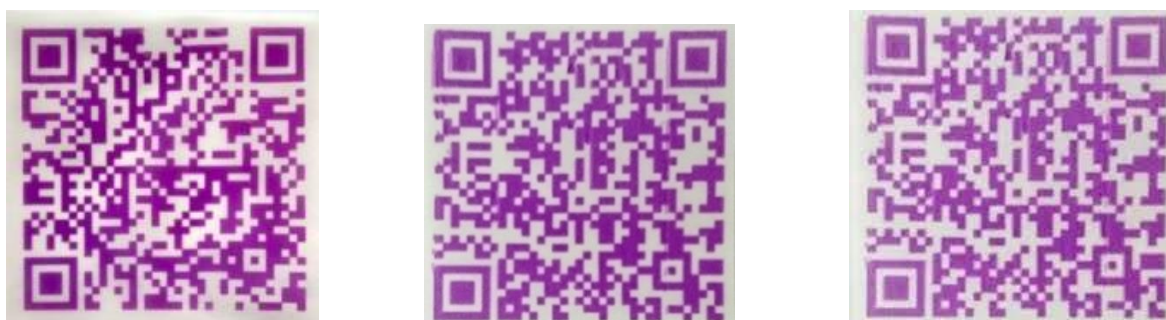
(A) QR code after printing (B) QR code at 75% RH storage (C) QR code at 95% RH storage
