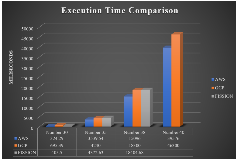
Figure 6.1: Execution Time Comparison between AWS, GCP, Fission
