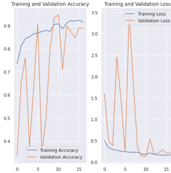
Figure 5.6: Training and validation accuracy and loss for 3-class (X-ray images)
