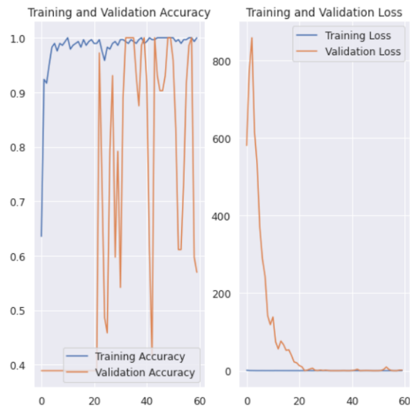
Figure 5.9: Training and validation accuracy and loss for 2-class (CT scan images)
