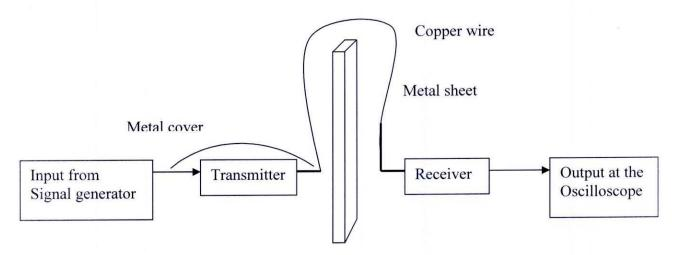
On connecting the antenna ports of the transmitter and the receiver the receiver end was now able to collect the signal directly and the output received was perfect like stage 1 and 2. The output obtained from the oscilloscope is as below.
