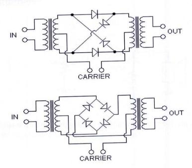
A balanced modulator is required to convert electrical energy into electromagnetic wave, preferably radio wave or microwave. We can implement the above circuit to bring about the desired conversion and utilize LM1596 integrated circuit.
