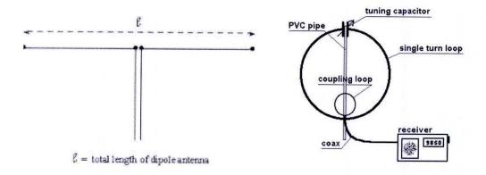
A dipole antenna is a radio antenna that can be made by a simple wire, with a center-fed driven element. The length of the antenna is inversely proportional to the frequency of the wave by a relation 147/frequency. Hence, greater the frequency, smaller is the size of the antenna, resulting in a more feasible and practically useful device.
