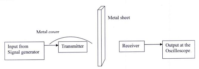
During the experiment, a metal sheet of steel was placed between the transmitter and receiver set up. And besides this metal obstacle, the transmitter was also covered with a metal case to stop any kind of data being transmitted. And there was no signal received at the output. The output at the oscilloscope is shown below.
