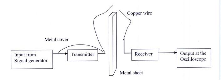
And then, after cutting the connecting wire into two halves, the antenna ports were connected to small wires of definite length that acted as wire antennas.
