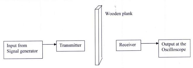
The wooden plank did not alter the transmitted data and the data signal received by the receiver modem was perfect as shown below.
