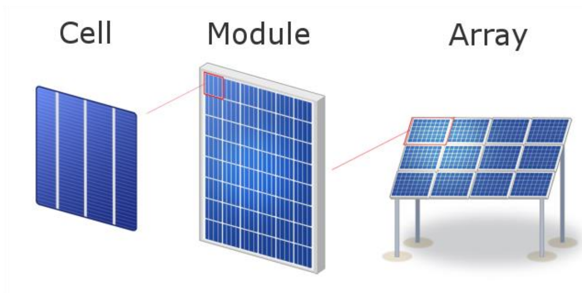
Figure 3.1.1: Solar cell, PV solar panel, and PV panel array
