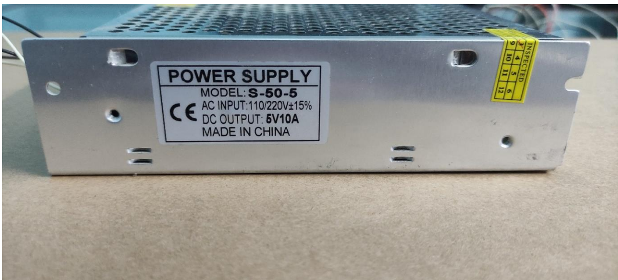
Figure 4.10: Power Supply (5V10A)
