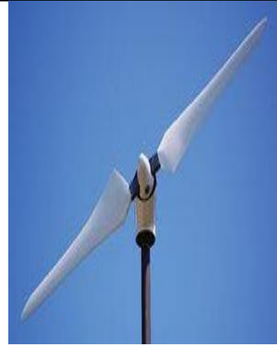
Figure 2.7.2: Two Bladed Horizontal Axis Wind Turbine [15]
