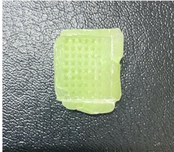
Figure 8 Wax fabricated mold prototype
