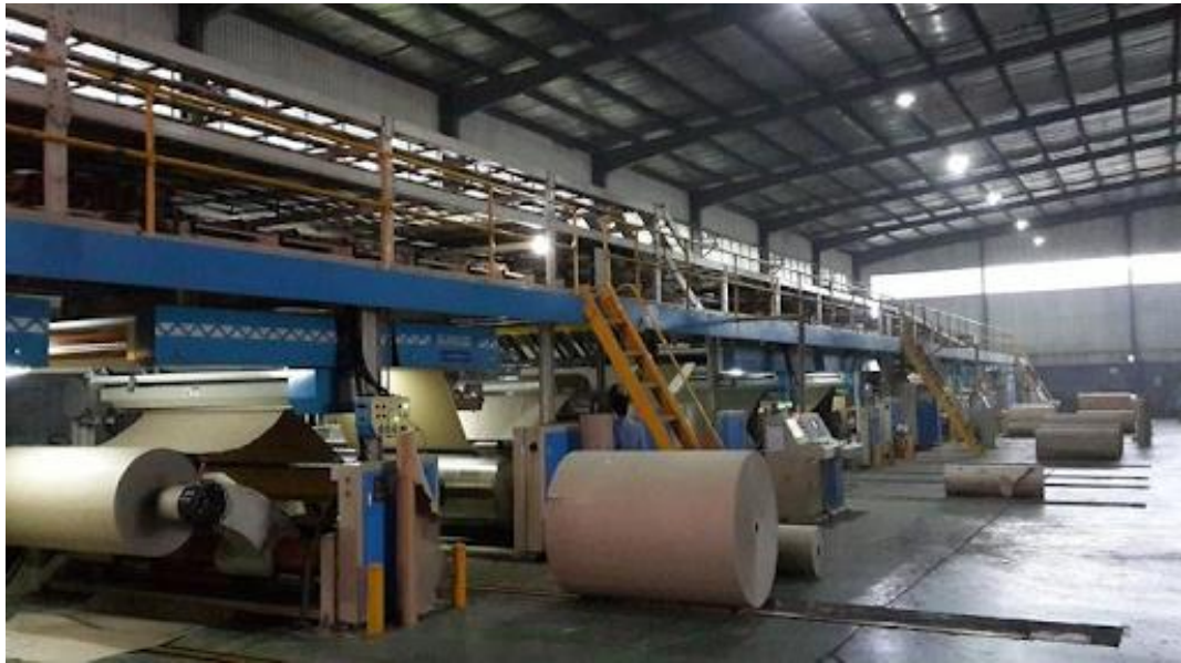
Picture 2: Automated Carton making machine.
