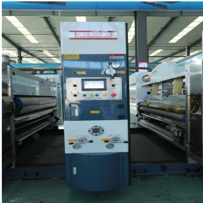
Picture 1: Dashboard of automated carton making machine.
