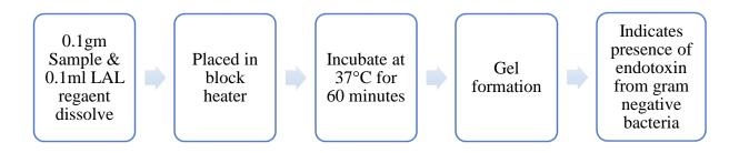
Figure 32: LAL Test process
