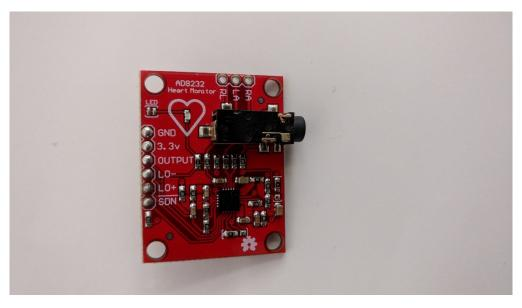
Figure 4.3: AD8232 Heart Rate Sensor
