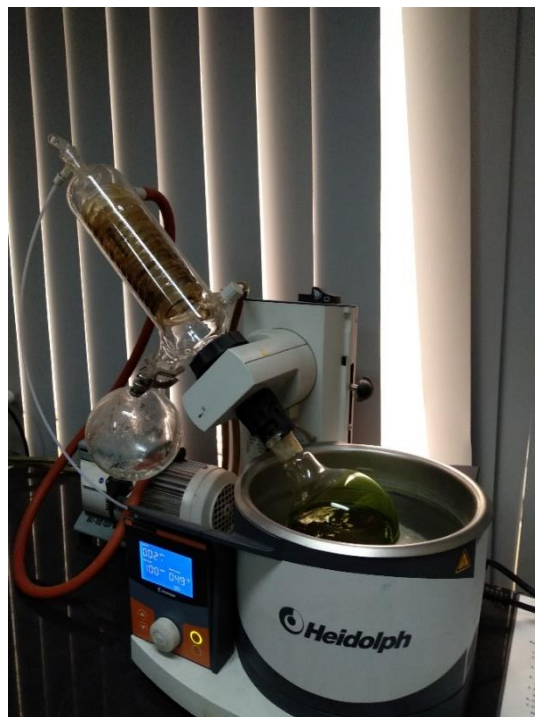
Figure 10: Rotary Evaporation of dissolved plant materials in methanol
