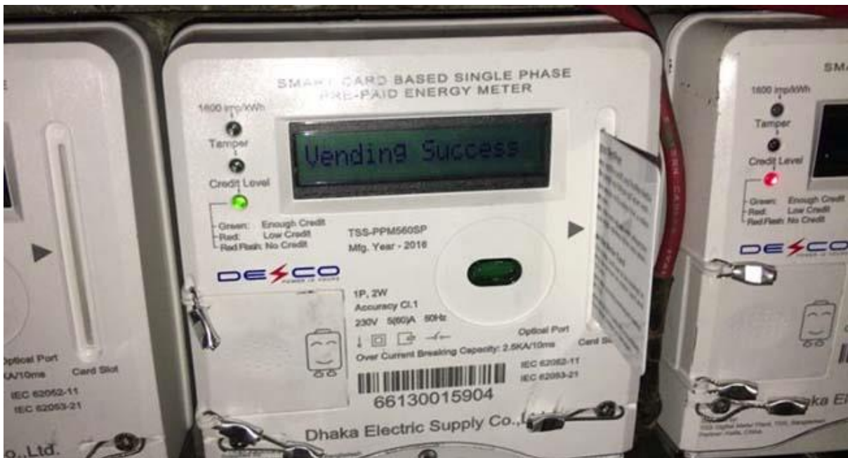
Figure 2.10: A digital Prepaid Meter used by DESCO, being recharged by a consumer.
