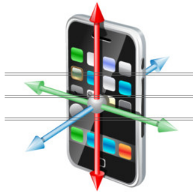
Figure 3.2: Smartphone and accelerometer axis
