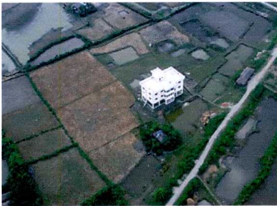
This cyclone shelter lacks a proper approach with the road and is isolated from settlements (source: http://www.sullivan.net/ )
