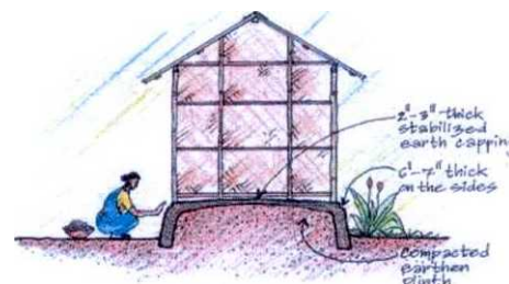
Mud stabilization of plinth
