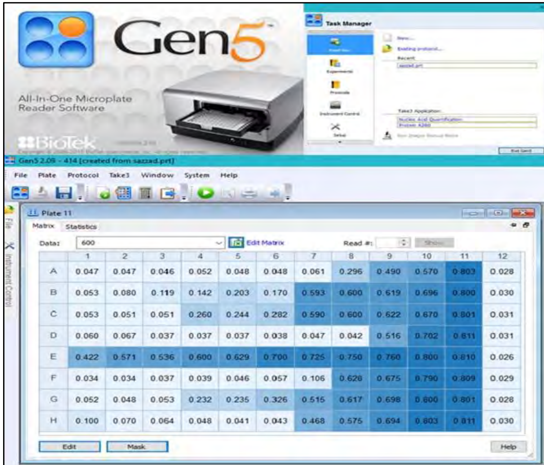
Figure 3.21: Minimum Inhibitory Concentration (MIC) data analysis Picture; result was determining in Nanoplate with the help of GENE 5 2.09 software. 11 th column is free from antibiotic and 12 th column free from antibiotic and bacterial inoculum.
