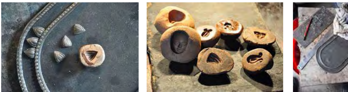
Figure 8: Sprig moulds for lost wax method (Source: Dhamrai Metal casting, Making Space: Sensing Place, Steven Follen)
