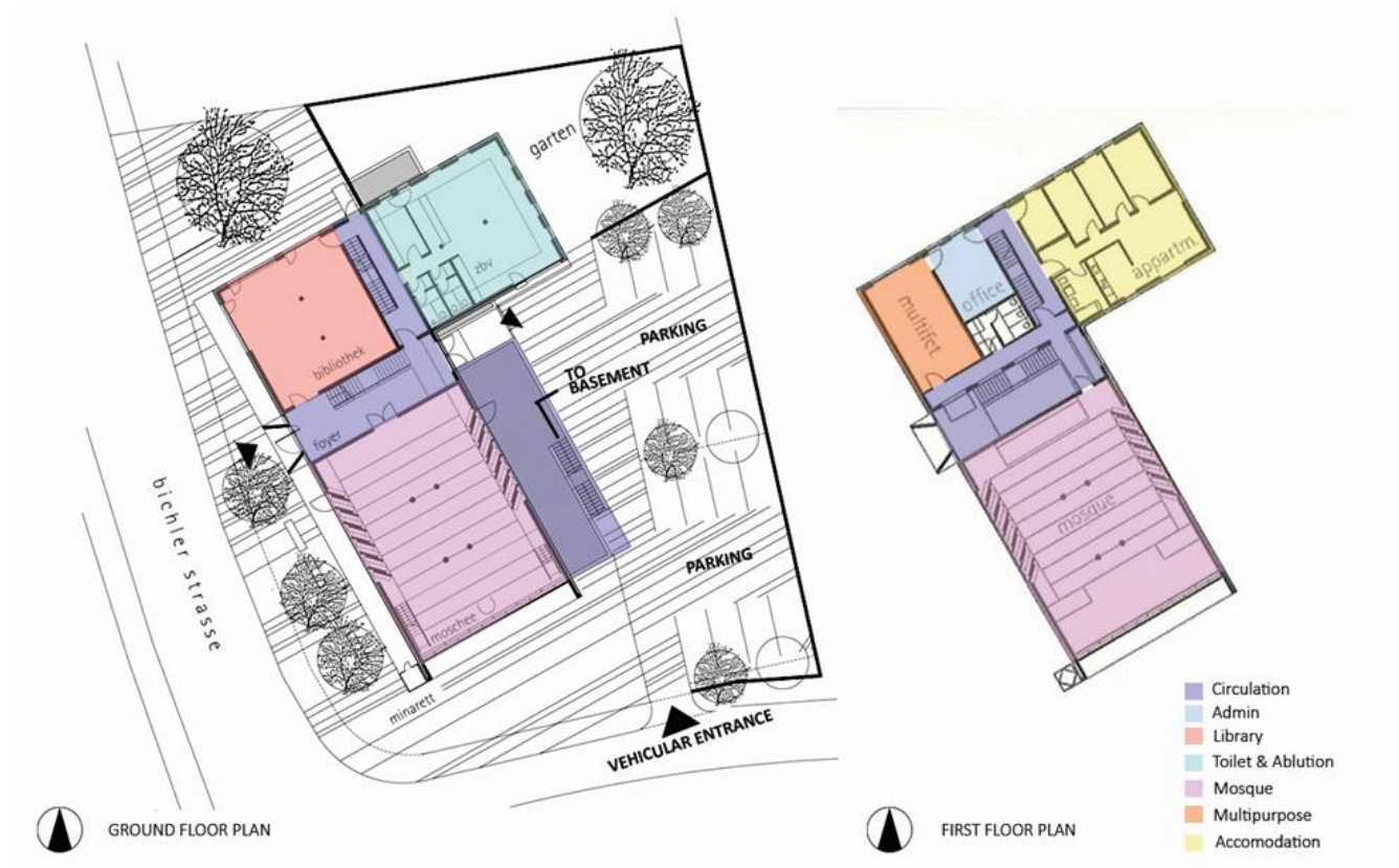
Figure 84: Ground floor plan and first floor plan. Source: Author (labelling); Plans adapted from ARCHITECT'S RECORD 2010 AWARD CYCLE, 2010, 3521. GER
