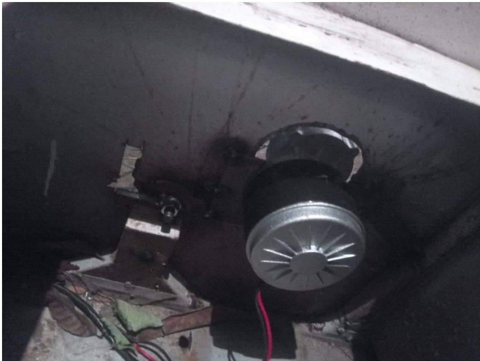
Figure 21: BLDC Motor mounted inside wheelchair
