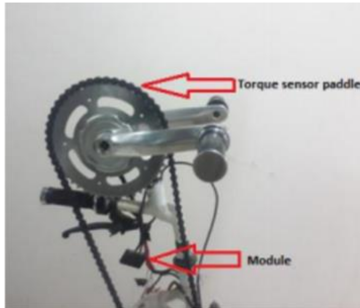
Figure 35: Torque Sensor pedal and module installed in the vehicle
