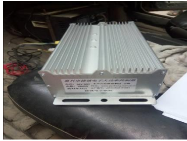
Figure 3.1: Upgraded Motor Controller.
