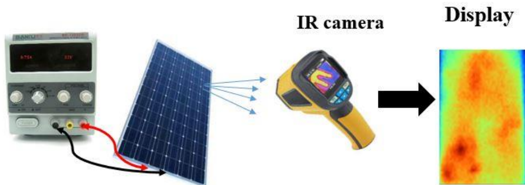
Fig. 2.5: Process of having infrared image of PV modules
