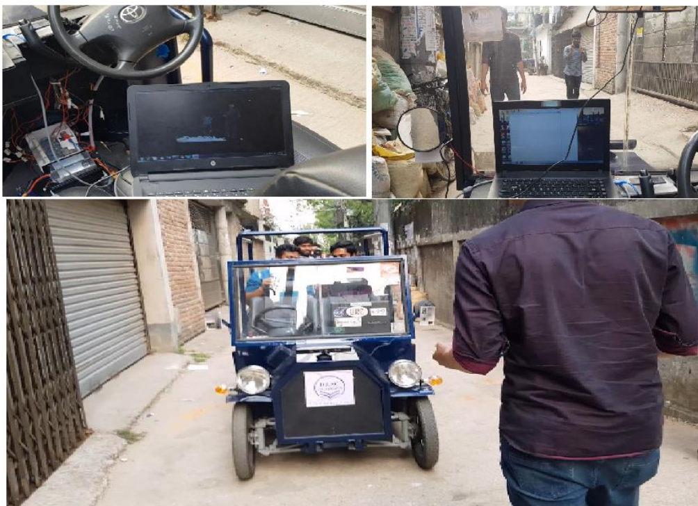
Fig.5.1. Obstacle avoidance using Kinect and sensor node
