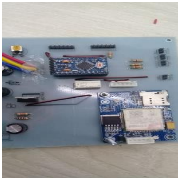
Fig.3.15. Developed Node – 3 module for CAN Bus network
