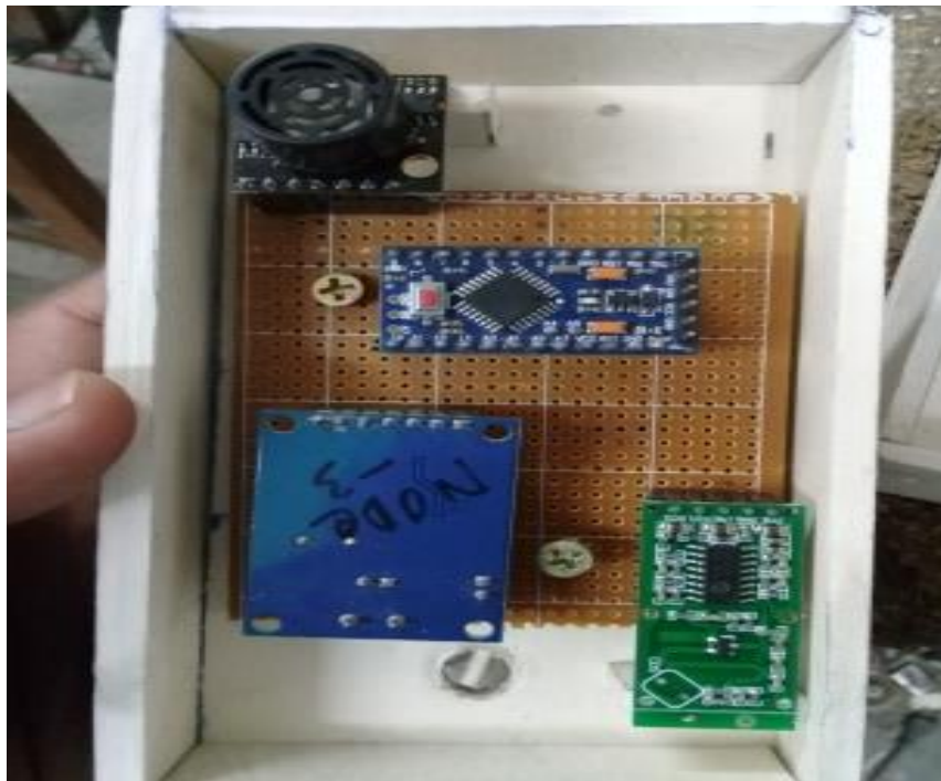
Fig.3.14. Developed Node – 2 module for CAN Bus network
