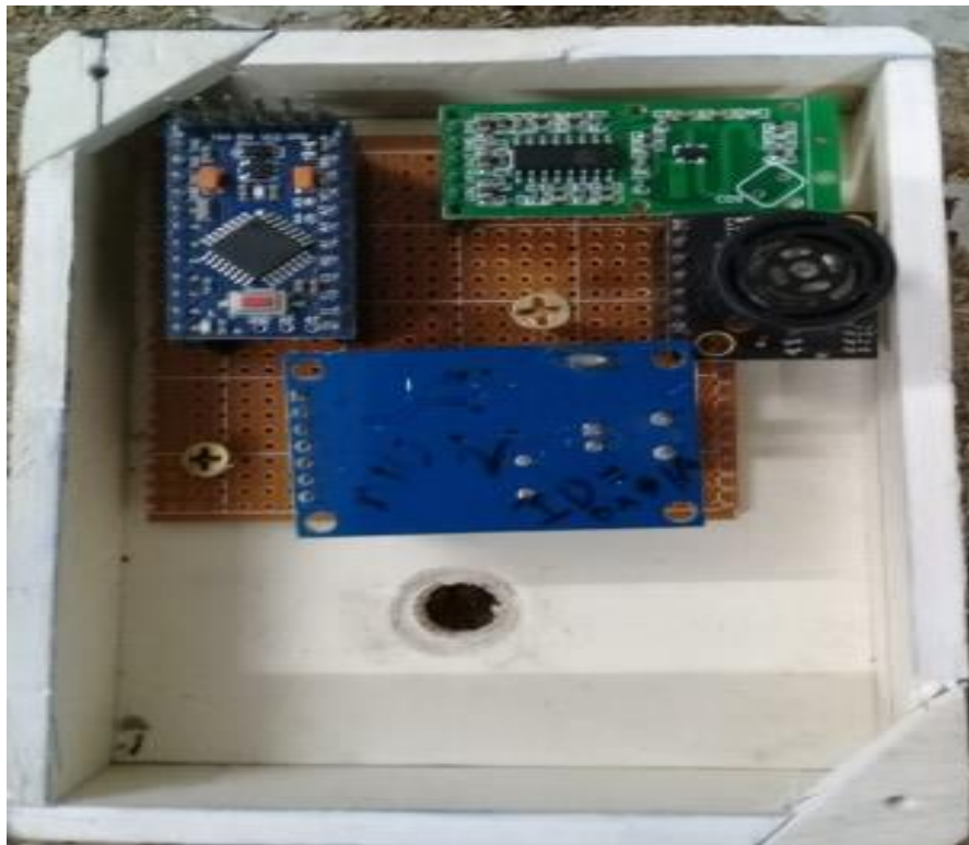
Fig.3.13. Developed Node – 1 module for CAN Bus network
