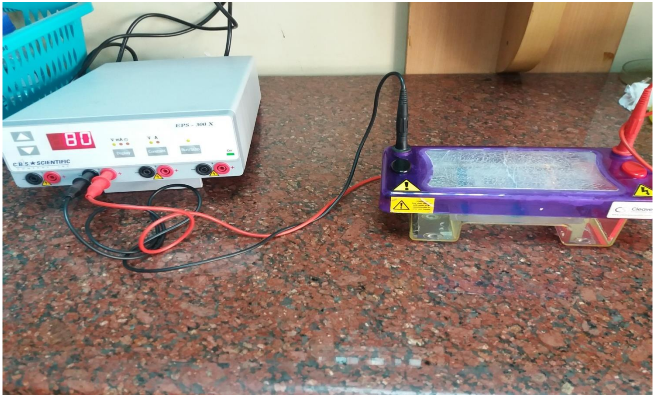
Figure 1.9: Gel electrophoresis apparatus
