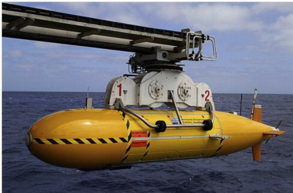
Figure: 2.2a The UK Natural Environment Council (NERC) Autosub6000 AUV [24]
