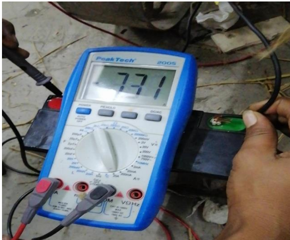
Fig 4.32: Glass motor (cutting blade) current at approximate load.
