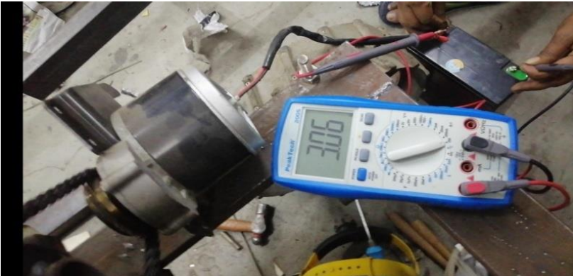
Fig 4.30: Measuring Cycle motor (Threshing drum) current at approximate load.
