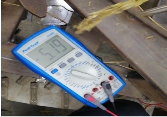
Fig 4.31: Measuring Cycle motor (Chain line) current at approximate load.
