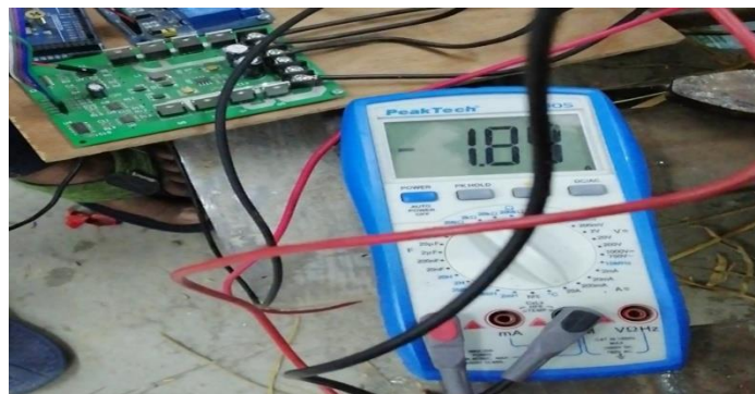
Fig 4.33: Measuring Wiper motor (Push-in gears) current at approximate load.
