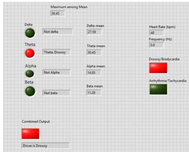
Figure 5.5.4.1: Front Panel giving a Confirmed Output by Combination of Signals
