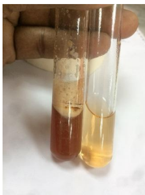
Figure 3.8: Addition of nitrate reagent. Nitrate negative
