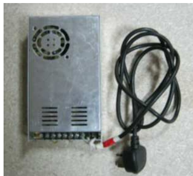
Fig. 2.13: 24-volt DC power supply [2].
