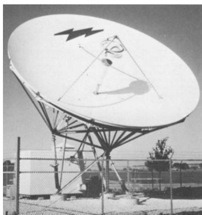
Figure: 6 Parabolic Antenna [6]
