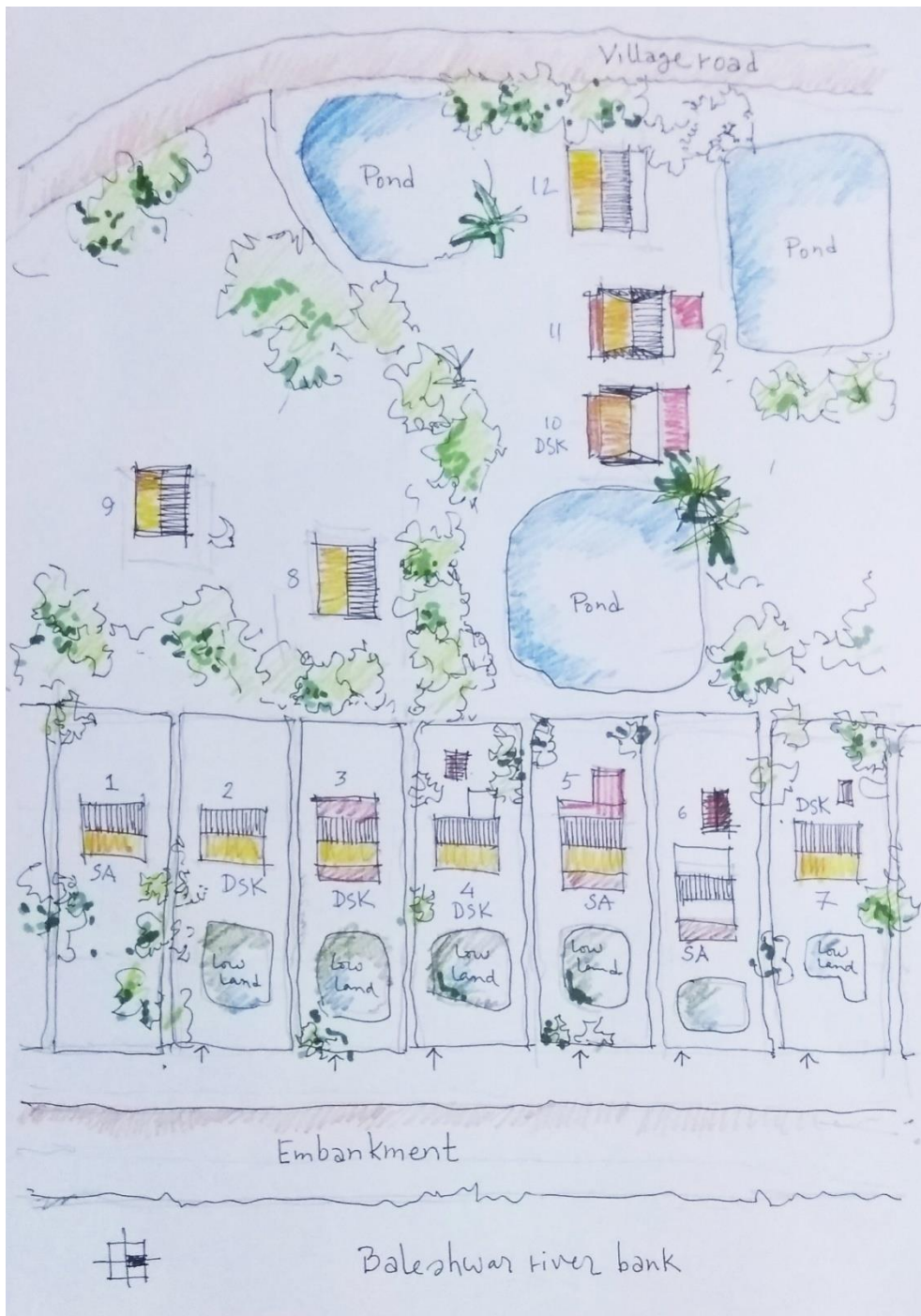
Fig. 5.18: Relocated settlement in Uttar Southkhali village beside the embankment of Baleshwari river. These lands were purchased by the distressed families from their relatives and neighbors in a row housing like pattern resulting in a settlement somewhat alien to the existing landscape. The dig and build process was used to raise the land and bhita. Some fallow low land (unsuitable to be ponds) beside the embankment lay unused. Trenches also run along the sides restricting movement between neighbors typical in rural setting.
