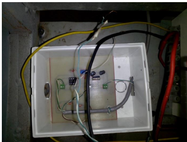
Fig 4.8: Torque adjustor circuit inside the wheelchair
