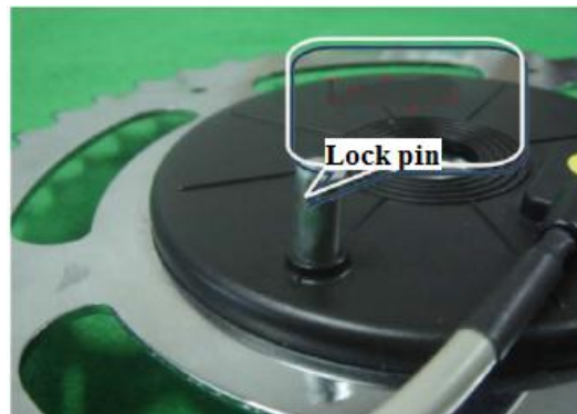
Fig 4.3: Lock pin at the back of the sensor
