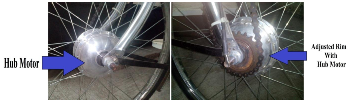
Fig 2.5: Hub Motor & Adjusted Rim
