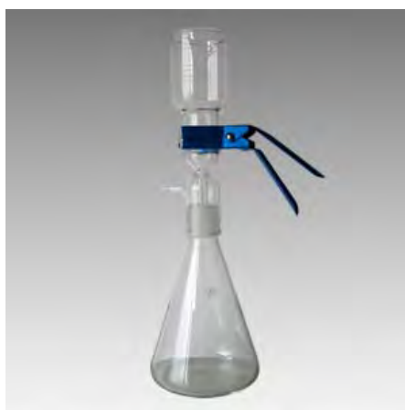
Figure 2.2 Vacuum filtration unit (HPLC)
