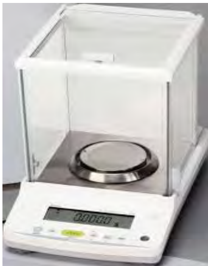
Figure 2.5 Electronic Balance, Model: (ATY 224), Shimadzu, Japan.
