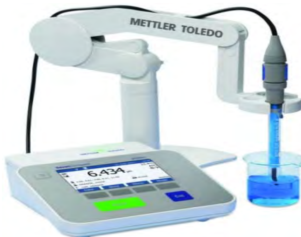
Figure 2.4 Digital pH meter bench top, model: (S220).
