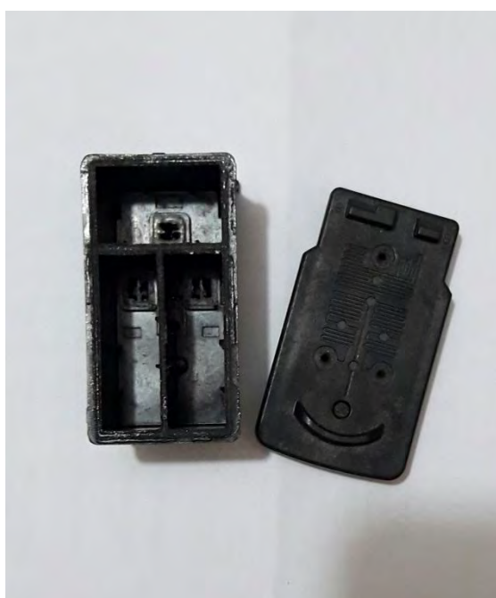
Figure 2.6 B: Inside of tricolor cartridge after cleaning
