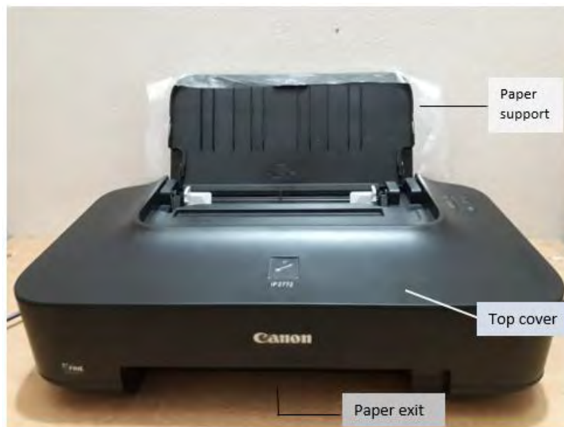
Figure 2.3: Different parts of Canon PIXMA ip2772 thermal inkjet printer
