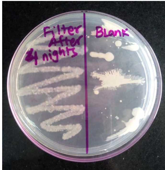
Fig 4.1.6 Growth of bacteria in water treated with charcoal and left for 4 nights observed in agar plate.
