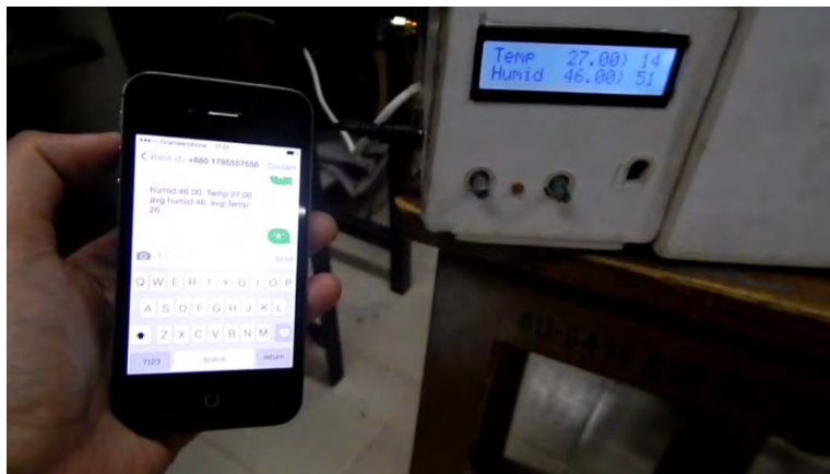
Figure 4.7.2(a): The GSM Module sent message to the user
