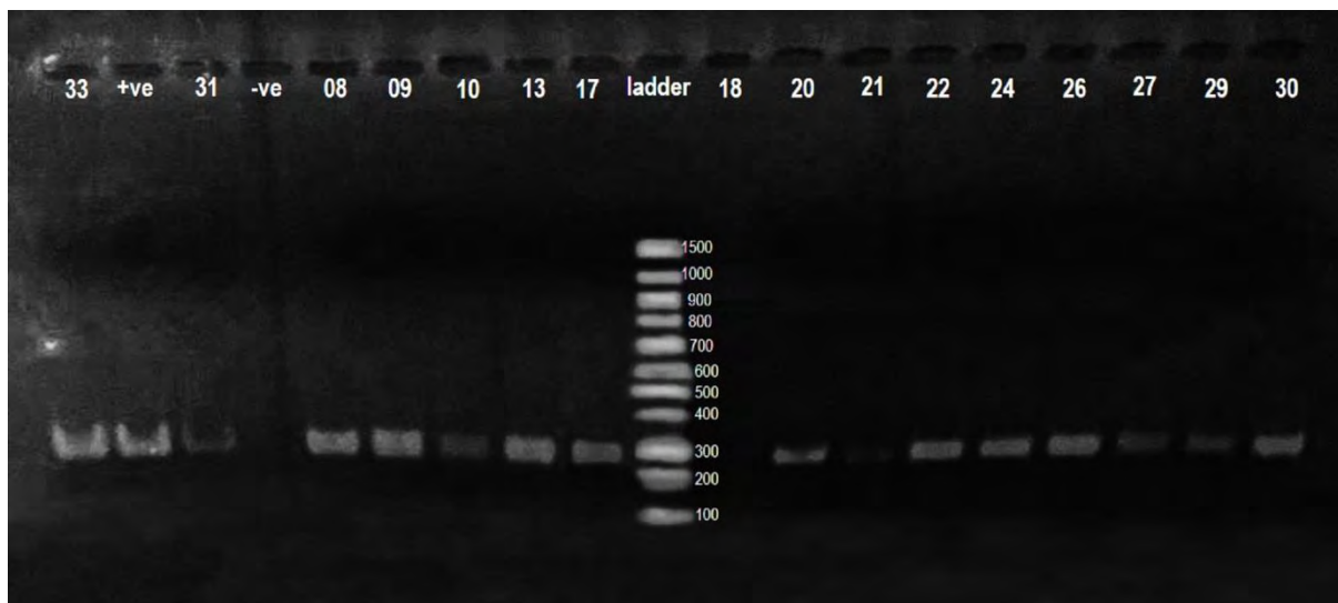
Figure 5: Agarose gel electrophoresis of isolates from Hatirjheel Lake showing positive bands for primer specific invA gene.
