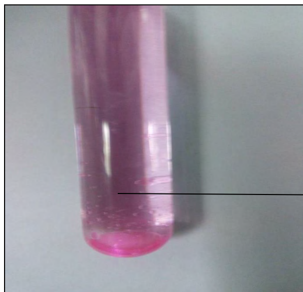
Figure 8: After ultrasonication, the oil in water emulsion
